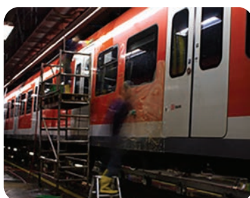
Step 2: Intensive cleaning with Transolv.
