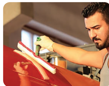
Step 12: Applying the permanent coating - Permaseal TP.
