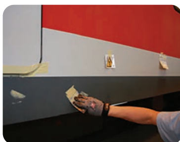
Step 5: Filling of paint chips with special 2k polyester filler.
